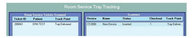
Users are able to see the tickets that are scanned and view what tracking point they have been scanned at. The right hand portion shows what scanners have been checked out and what track point a current user is at.
